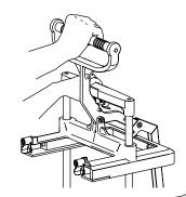
Holding the pusher and blade components together as one cartridge, remove from the chassis. Guide the sides of the pusher component out of the C-shaped channel in the chassis.
