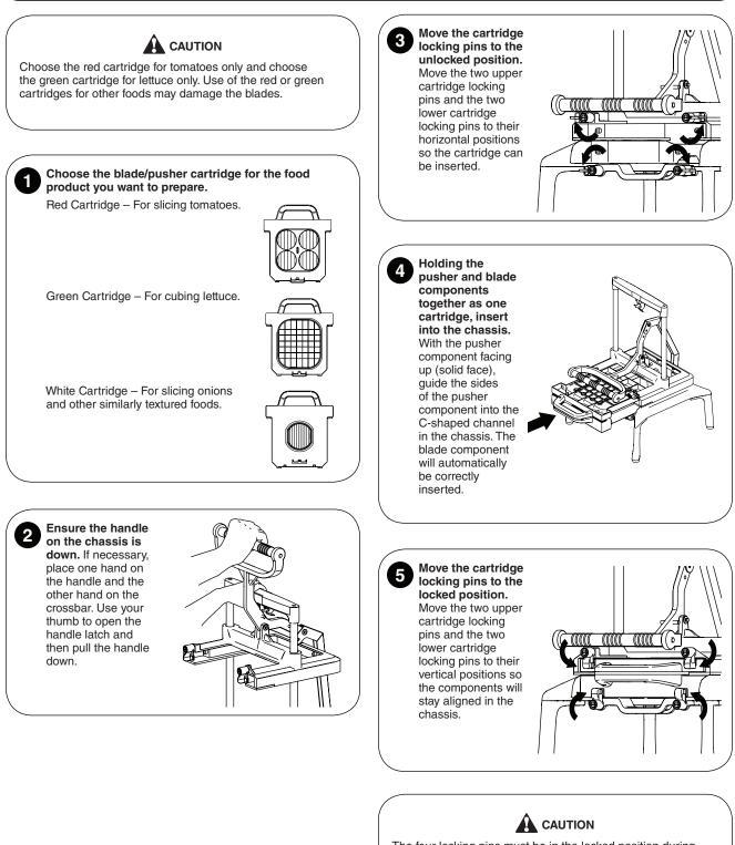
The four locking pins must be in the locked position during operation to prevent damage to the blades.
