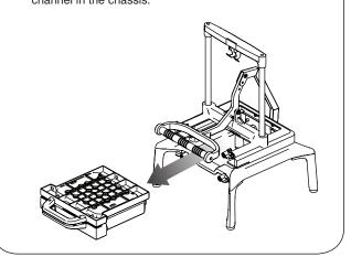
Move the cartridge locking pins to the unlocked position. Move the two upper cartridge locking pins and the two lower cartridge locking pins to their horizontal positions so the cartridge can be removed.
